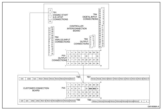
Figure 6-6 Controller (Customer) Connection Kit
